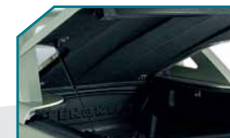
▶ Easy opening with superior quality Gas Struts.
